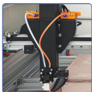
Dual feeder single nozzle for multi-color
